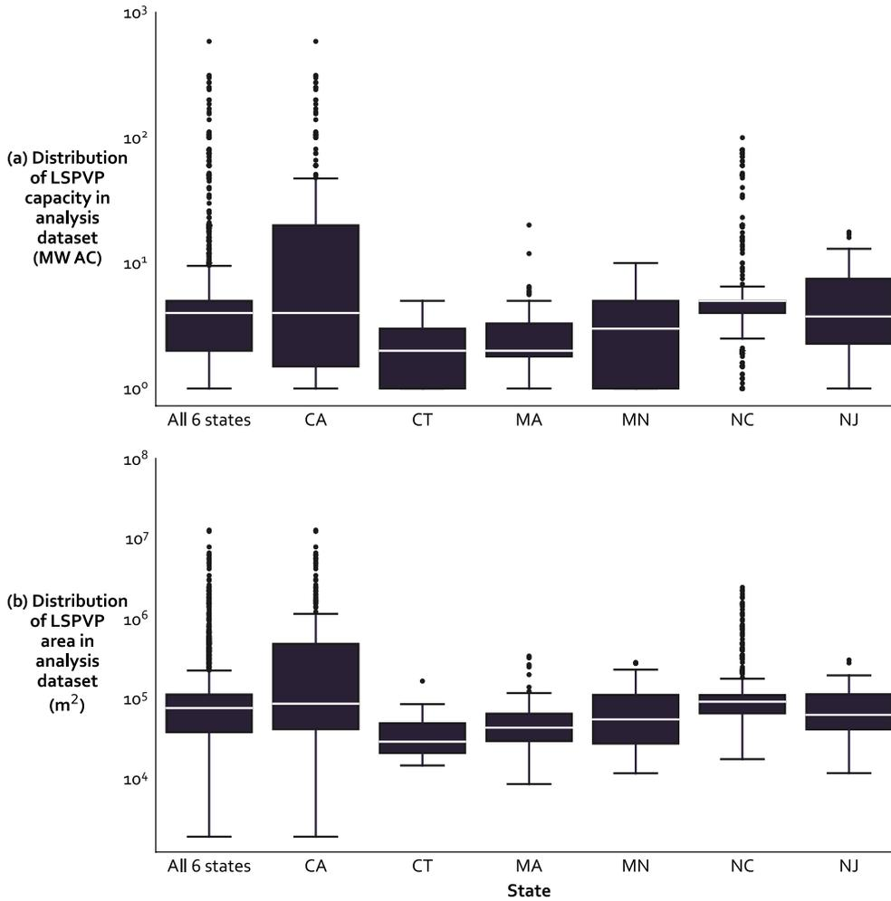
Fig. 5. Distribution of (a) capacity in MW AC and (b) ground-mount area in  $m^2$  of unique LSPVPs in analysis dataset by state. Line represents median value; box limits represent 1st to 3rd quartiles; whiskers represent 4x the inter-quartile range.
